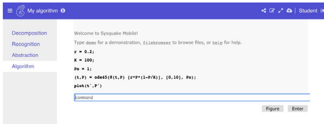
Figure 14. Commands for the simulation of the evolution of a population with Sysquake.
